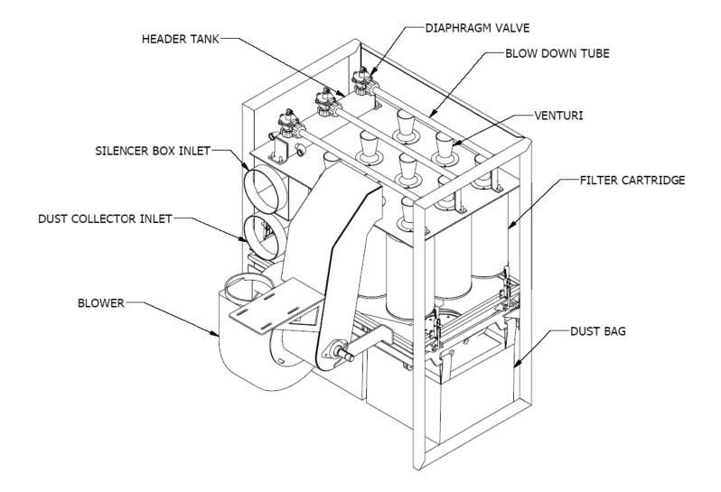
**FIGURE 5: Dust Collector Components**
