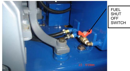
Figure 1: Fuel Shut-off Switch
